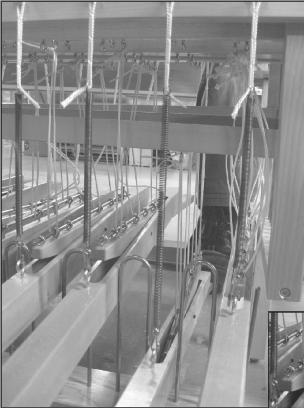
View from the back of the loom showing treadle #2 depressed with the treadle spring under tension.
